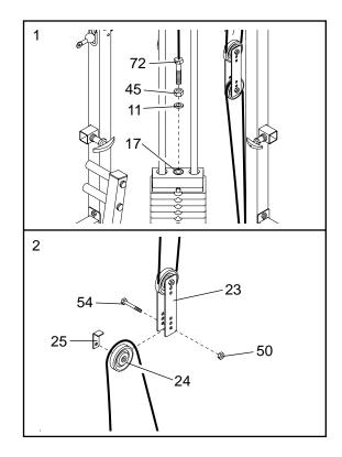
Do not overtighten the cables. If the cables are over tightened, the top weight will be lifted off the weight stack. If a cable tends to slip off the pulleys often, it may have become twisted. Remove the cable and re-install it.
